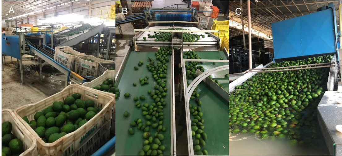
Figure 1 - Avocado packaging house - Harvested fruit (A); Conveyor table reception (B); Cleaning (C). Source: Jaguacy Avocado Brasil.
